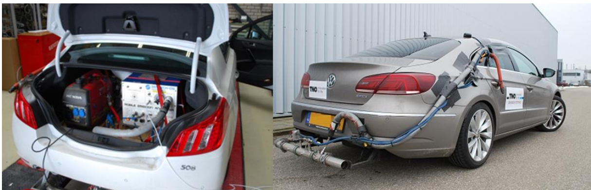
Figure 12: The PEMS system mounted on vehicles to be tested on the road
