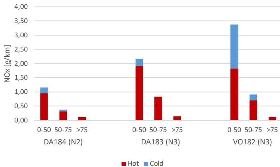
Figure 8: Contribution of cold starts in total emissions per speed interval: NO<sub>x</sub> emissions when the engine has a coolant temperature <70 °C (Cold) and ≥ 70 °C (Hot).
