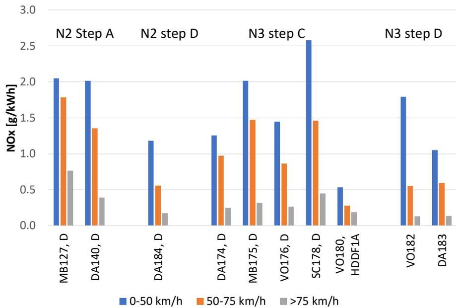
Figure 6: Overview of real-world NO<sub>x</sub> emissions as measured with SEMS during daily operation for medium lorries and tractor semi-trailers, all with Euro VI certified engines (D=Diesel, HDDF = Heavy Duty Dual Fuel Engine). The vehicles with engines certified according different sub-class (Step A, C as tested in 2018-2019 and D) are shown together. Three speed ranges are distinguished. Individual vehicles can't be compared as operation differs from vehicle to vehicle.
