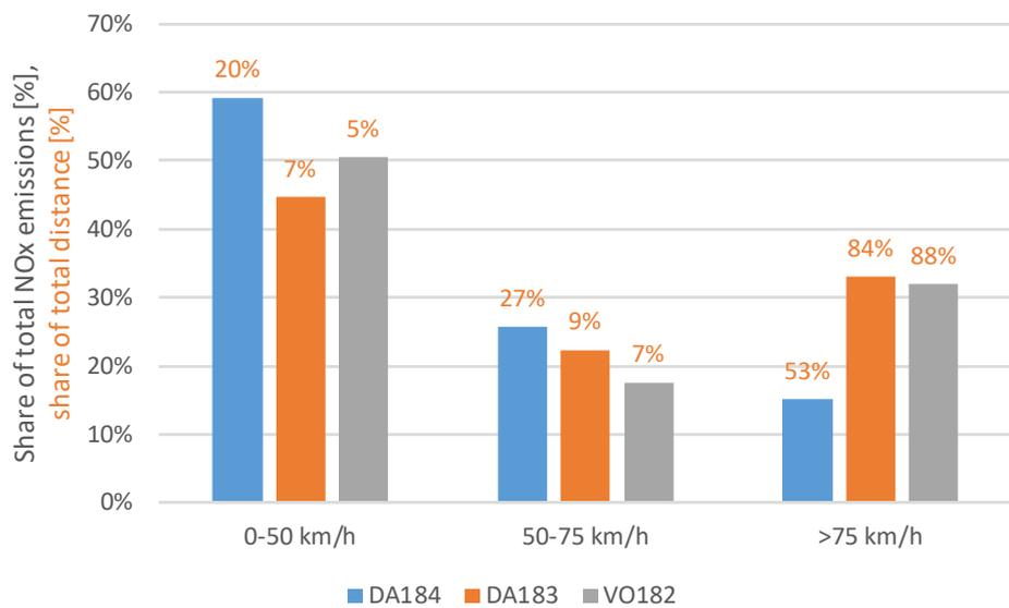
Figure 7: The share of the NO<sub>x</sub> emissions of the total emissions per speed interval of the tested vehicles with a step D certified engine. A large share of the total NO<sub>x</sub> (45 to 59%) is emitted at the low speed range whereas the most of the kilometres (53 to 88%) are driven in the higher speed range.
