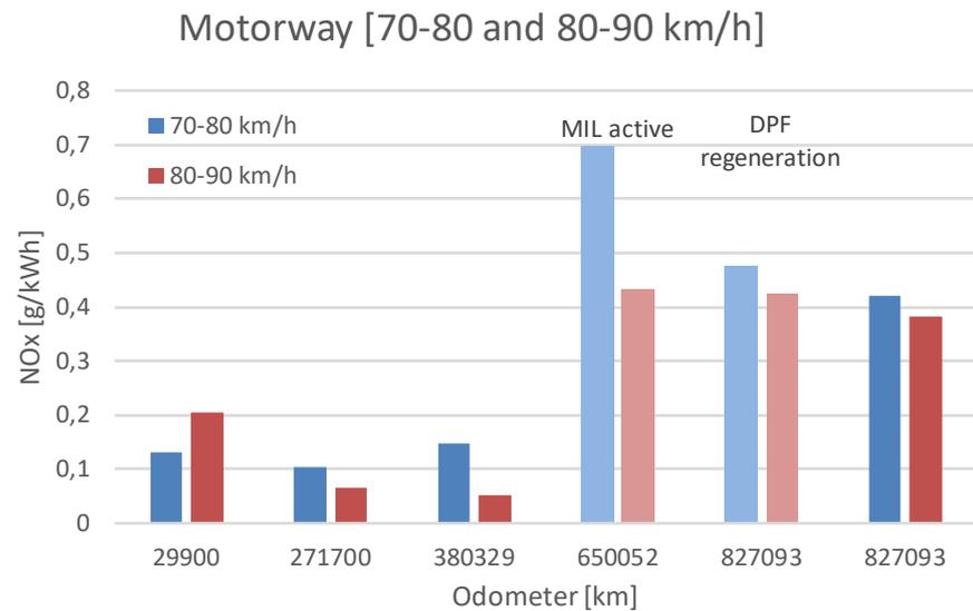
Figure 11: NO<sub>x</sub> in speed bins at motorway speeds. The trips have comparable motorway driving with a fully warmed up drive train and aftertreatment. Trips are driven with the same total vehicle weight (tractor, semi-trailer and payload).
