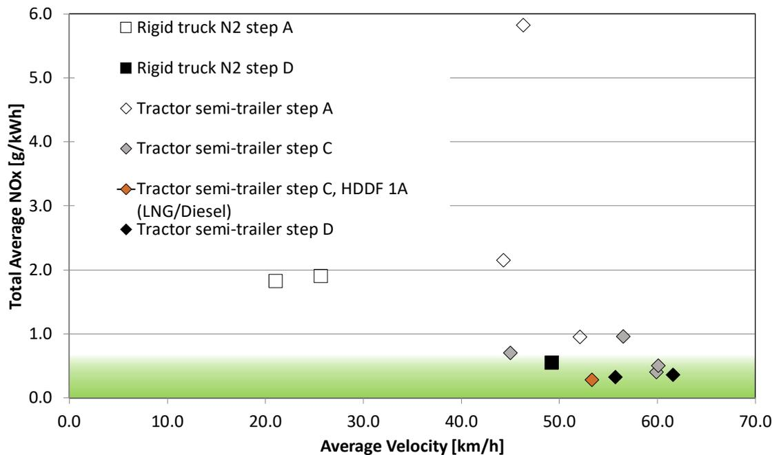
Figure 5: Total average NO<sub>x</sub> emissions versus average speed for all vehicles tested with SEMS in normal daily operation. The upper side of the green area represent a NO<sub>x</sub> emissions level of 0.69 g/kWh, which is the limit of the conformity factor of 1.5 expressed in gNO<sub>x</sub>/kWh ( $1.5 \times 0.46 = 0.69$  g/kWh) for the formal ISC test. Individual vehicles can't be compared as operation differs from vehicle to vehicle.
