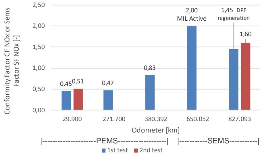
Figure 10: NO<sub>x</sub> conformity factors (PEMS) and SEMS Factors (SEMS) over N3 in-service conformity test routes at different mileages.
