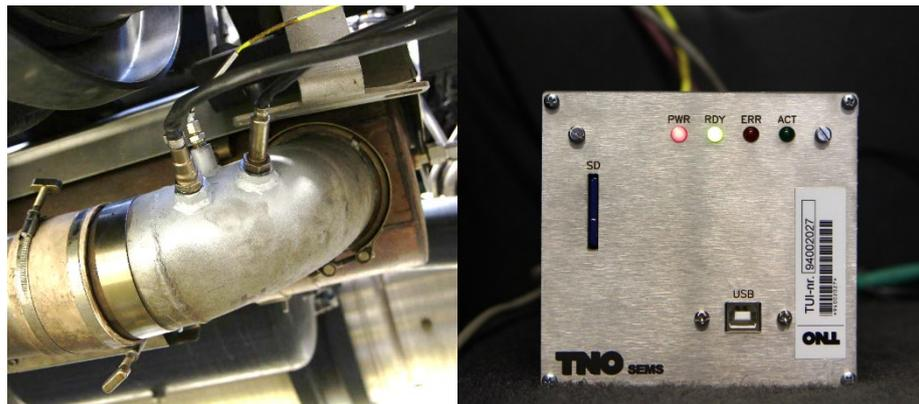
Figure 1: SEMS. *Left*: calibrated NO<sub>x</sub>-O<sub>2</sub> sensor, NH<sub>3</sub> sensor and temperature sensor mounted in the tail-pipe. *Right*: autonomously running data recording unit with hourly data transmission to a central server via GPRS.
