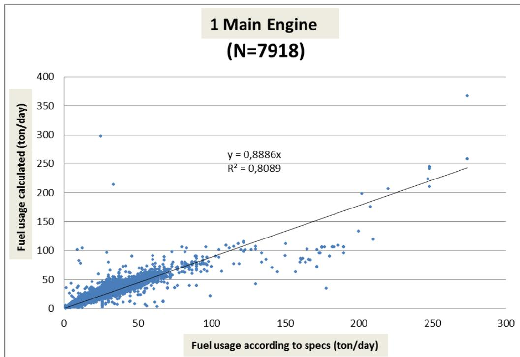
**Figure A-3** Calculated daily fuel usage of one-engine ships compared with specifications.
