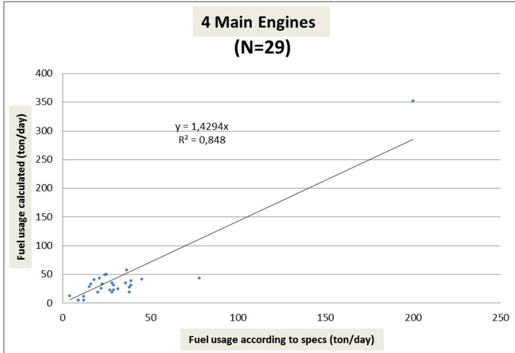
**Figure A- 5** Calculated daily fuel usage of four engine ships compared with specifications.
