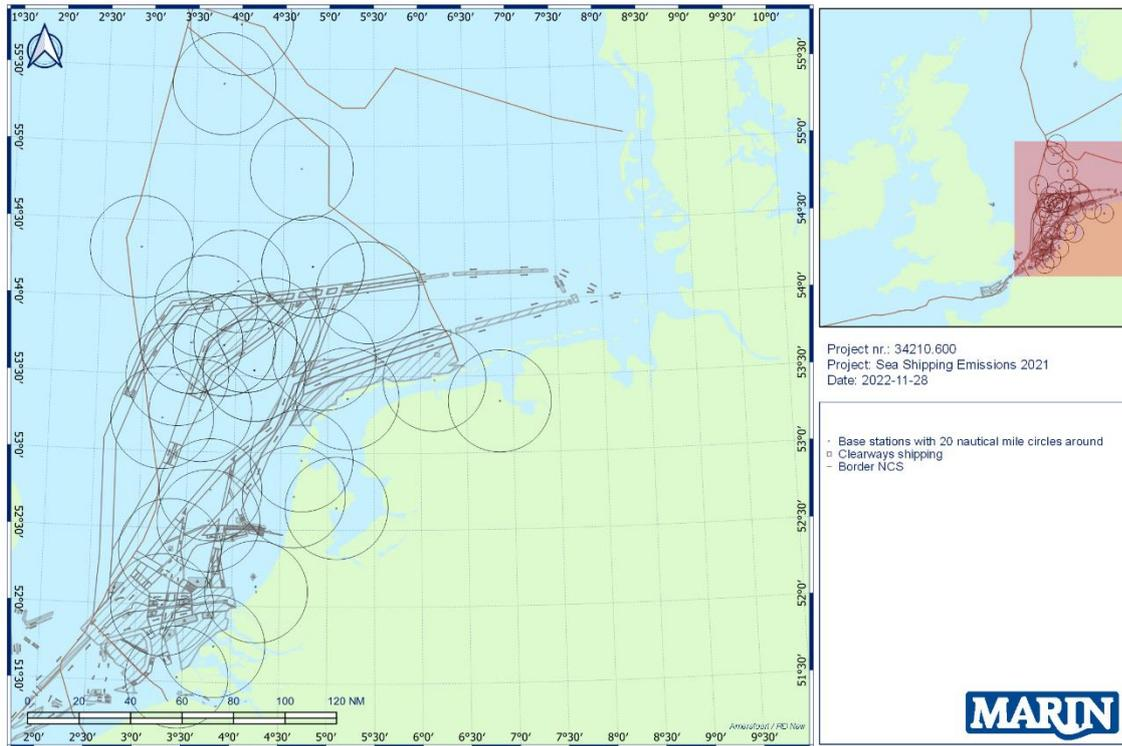
**Figure 4-1** AIS base stations in 2021 delivering data to the Netherlands Coastguard.
